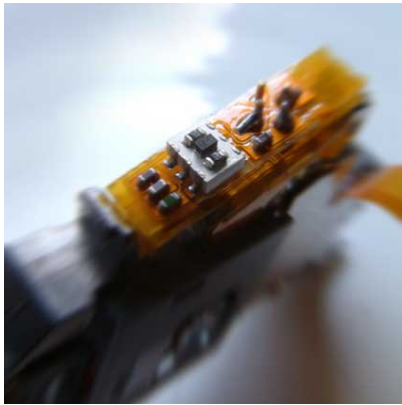
High-frequency superposed module installed in an optical pickup
